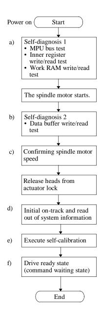
Figure 4.3 Power-on operation sequence
